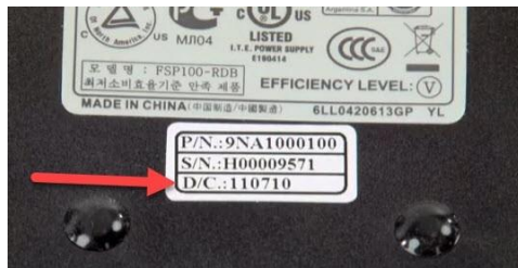
The above example shows a date code (D/C) of 110710
