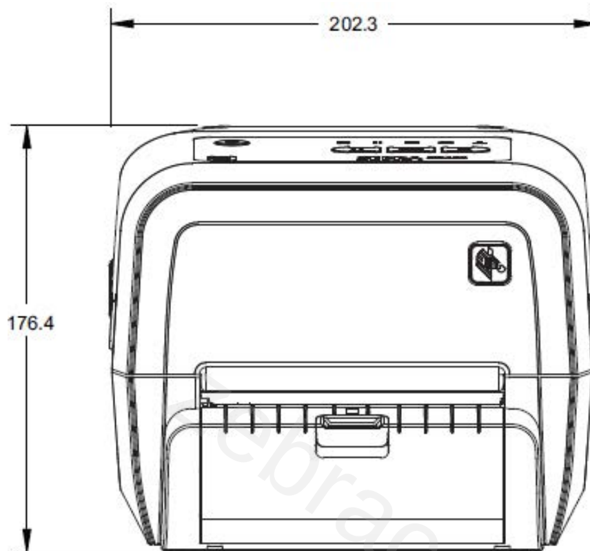
Figure 19 Ribbon Cartridge Thermal Transfer Printer with Label Dispenser (closed)
