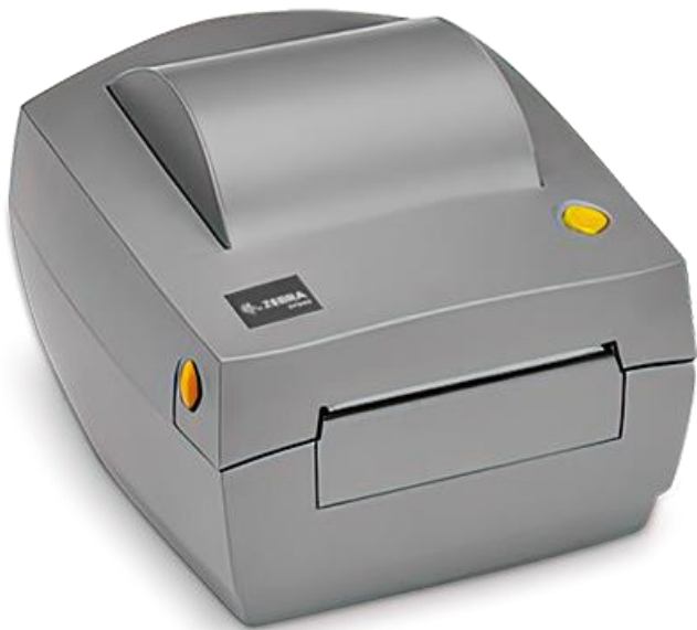
Entry-level 4-inch direct thermal label printer; not available in all regions
