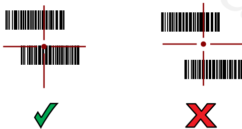
Figure 19 RS5100 Pick List Mode with Multiple Barcodes in Aiming Pattern
