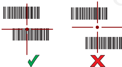
Figure 21 RS507/RS507X Pick List Mode with Multiple Barcodes in Aiming Pattern
