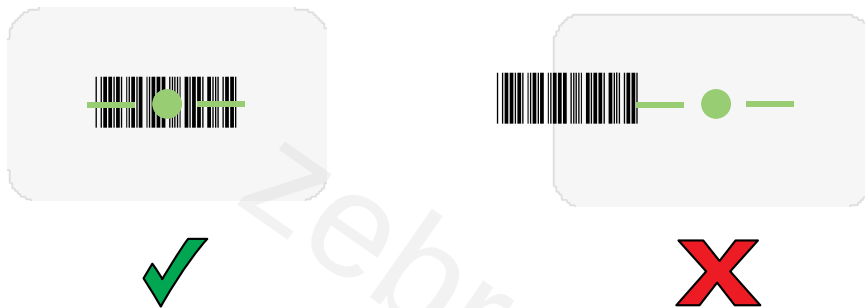
Figure 14 SE4720 Aiming for Pick List Mode with Multiple Barcodes
