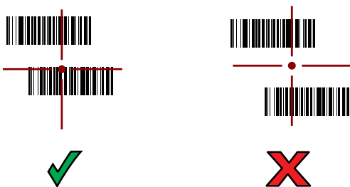
Figure 26 RS5100 Pick List Mode with Multiple Barcodes in Aiming Pattern
