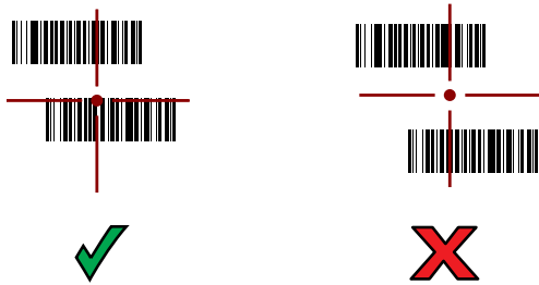
Figure 20 RS507/RS507X Pick List Mode with Multiple Barcodes in Aiming Pattern
