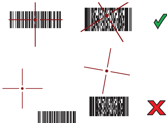
Figure 19 RS507/RS507X Aiming Pattern
