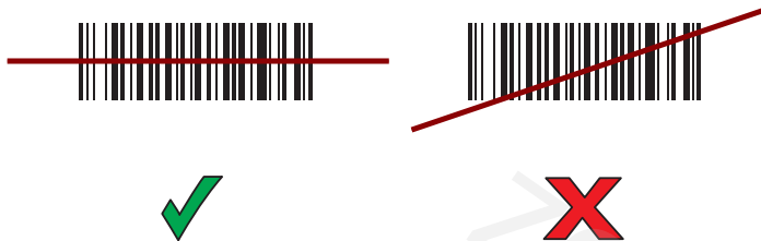
Figure 40 Laser Scanner Aiming Pattern
