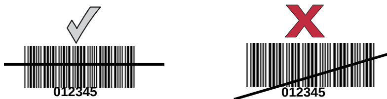
Figure 2-3 Acceptable and Incorrect Aiming
