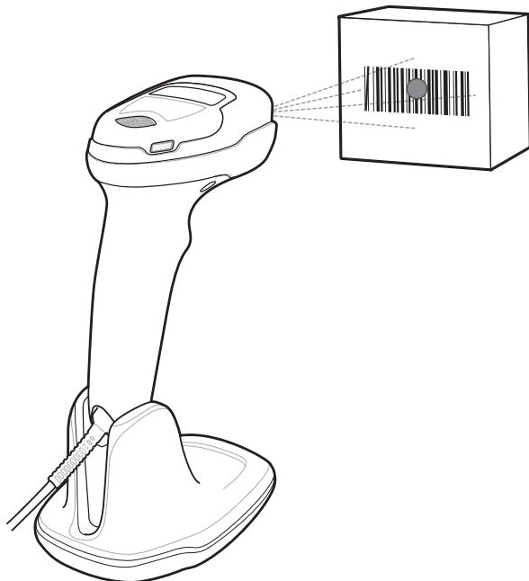
Figure 2-8 Scanning with the DS4308P
