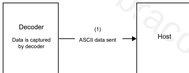
Figure 9-4 ACK/NAK Disabled and Unpacketed ASCII Data
