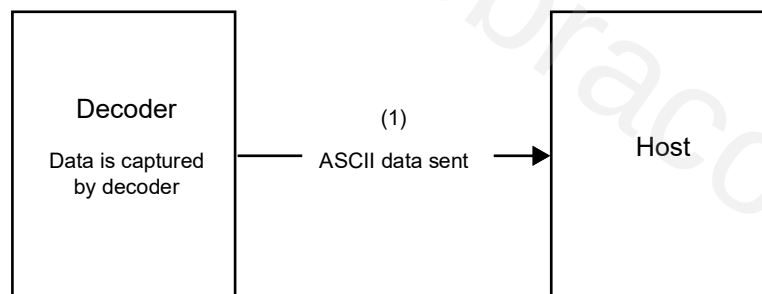
Figure 9-4 ACK/NAK Disabled and Unpacketed ASCII Data
